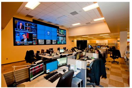
NEC's 7x4 video wall utilizes TileMatrix technology for a near-seamless look, along with a Swing Wall mounting frame and a unique failsafe imaging technology. © 2010 Ron Baker Photography
